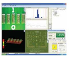
With ASC International's new ASCan Ultra measurement software, creating a fully automated inspection routine can now be completed in less than 10 minutes. In Run mode, the user loads the program, confirms fiducial alignment and the ASCan Ultra software automatically measures the Gerber imported programmed locations with a final "PASS" or "FAIL" message. A defect error review mode allows users to verify "Failed" locations and attach corrective action items for traceability.
