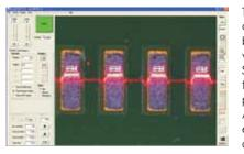
To obtain automated measurements on the **SP3D Mini**, position the circuit board under the system's laser-based vision sensor to the desired location. Simply click the large green run button to automatically calculate the solder paste height, width, area and volume. Automated measurements reduce the errors associated with operator to operator variations.
